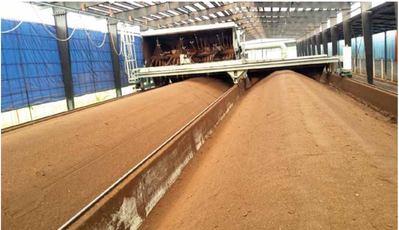
Composter machine above the compost pit at Kazi Raigonj Compost Plant of Kazi Farms Limited
